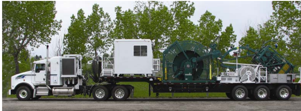
Coiled Tubing Unit
